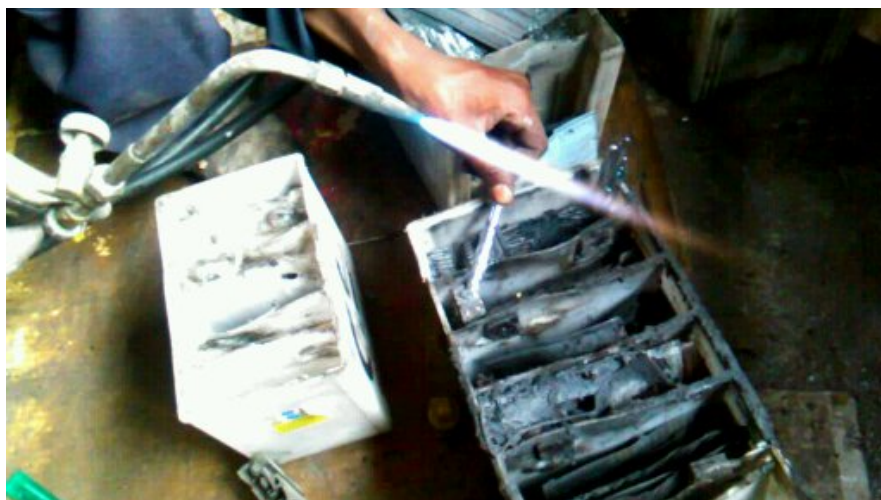
Figure- 2: Smelting of lead in a small scale LAB repair shop to join the two opposite poles.
